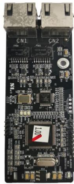
Ethernet/IP communication card STX510/ Modbus TCP communication card STX515
